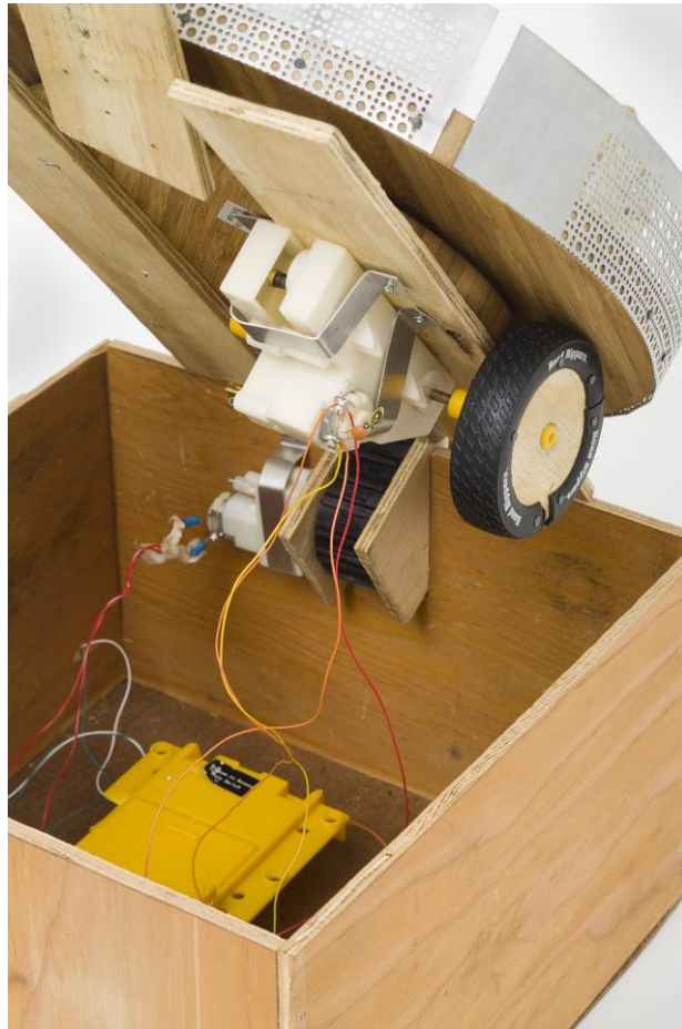
Fig. 8.39. The motor and method of rotating the Lazy Susan.
