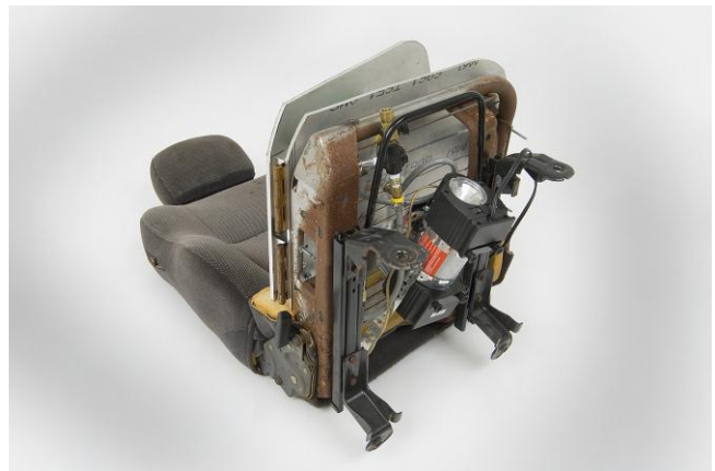
Fig. 8.77. Air compressor and hoses.
