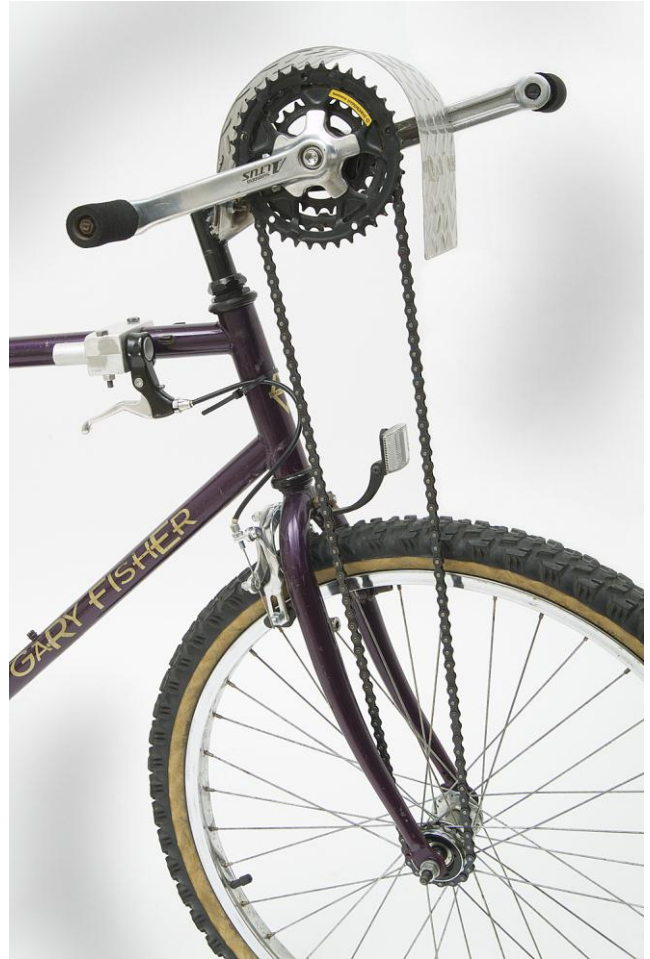
Fig. 8.93. Hand crank system with chain guard.
