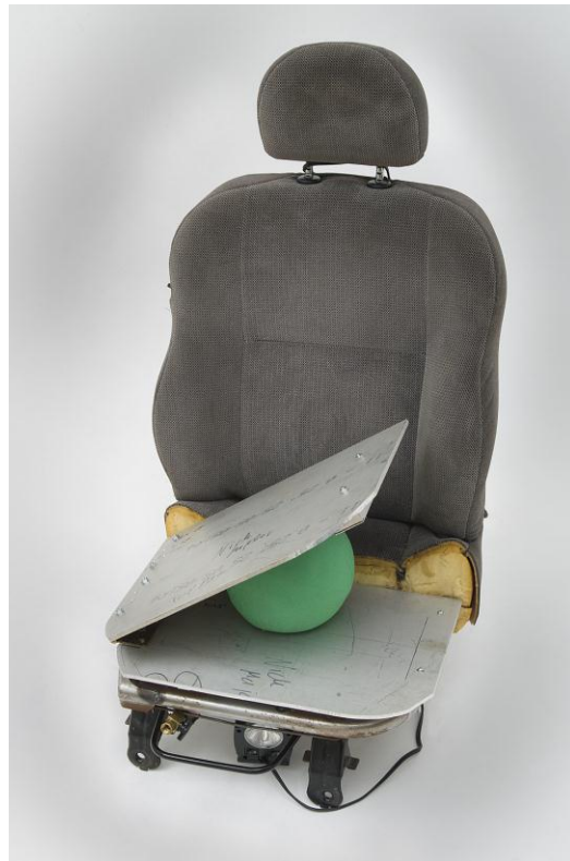
Fig. 8.78. Ball inflated lifting the seat.
